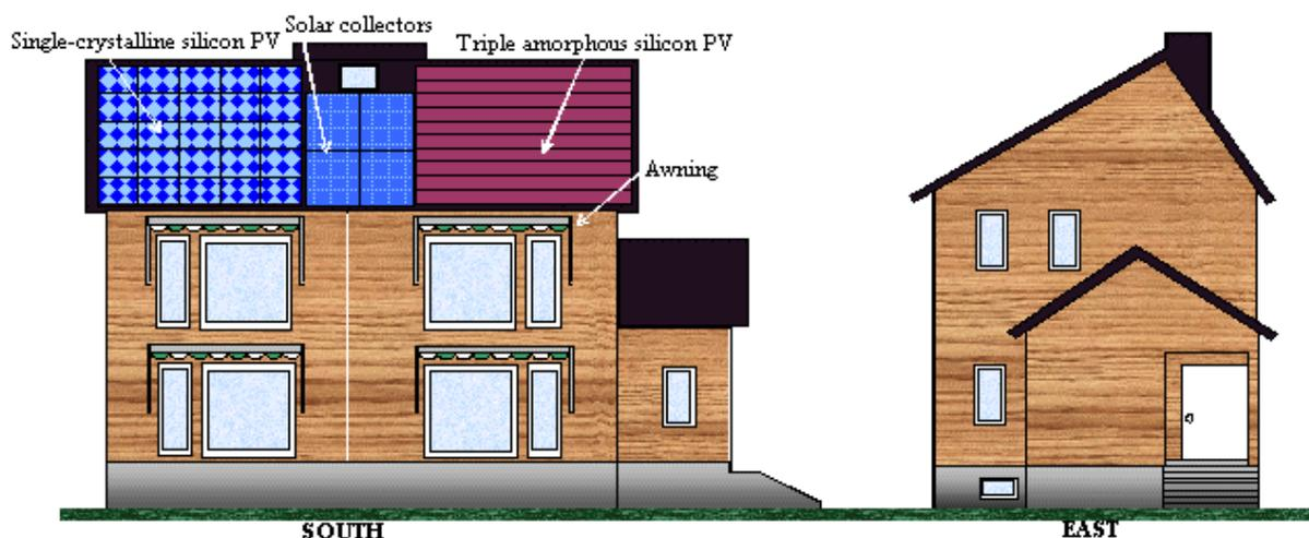
Fig. 1 Elevation of low energy house
