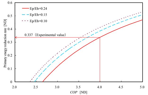
Fig. 6 Relation between COP of GSHP and primary energy reduction rate to typical heating
