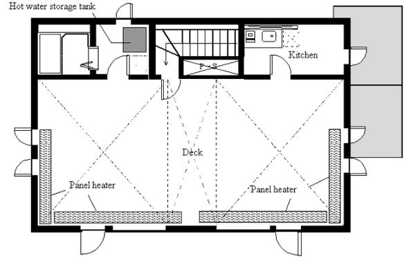
Fig. 2(b) The 2nd floor plan
